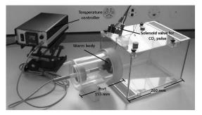
Fig. 1. The bioassay setup with the mosquito cage, warm body inserted into the port, temperature controller and solenoid valve for CO<sub>2</sub> pulse delivery.
