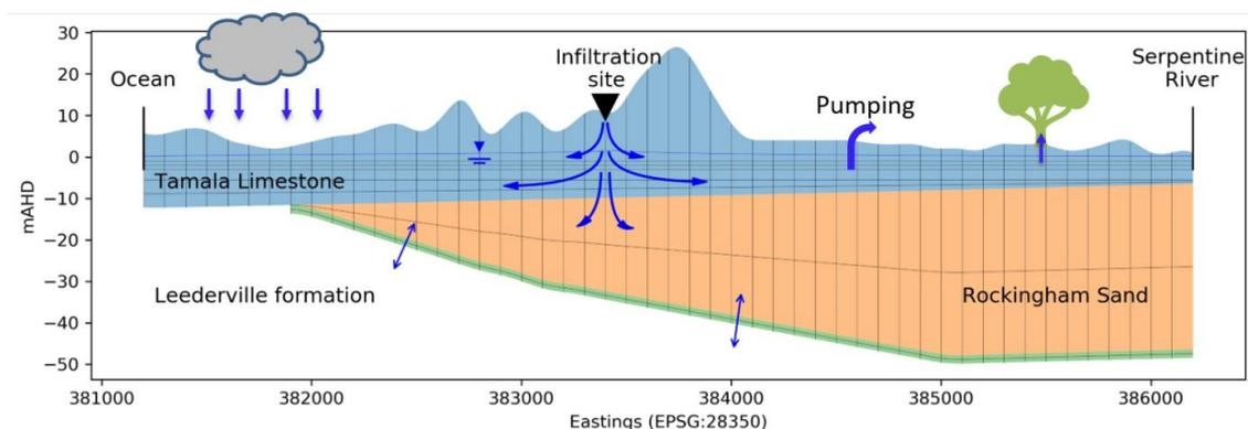
Figure 1: Conceptual model and model discretisation in a West-East cross-section view. The green layer is the fictive layer where boundary conditions between the Leederville formation and the Rockingham Sand are set. Note, there is no interaction below the Tamala Limestone. The wastewater infiltration site is the only source for carbamazepine, sucralose and the wastewater similar isotopic signature in the model.
