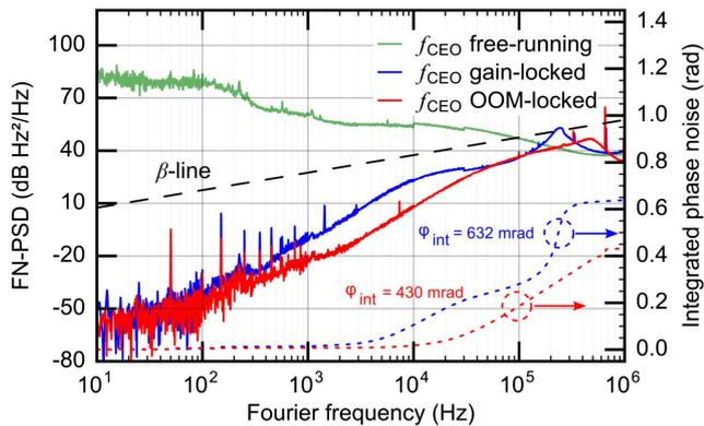
**Fig. 4.** Frequency noise power spectral density (FN-PSD) of the CEO beat obtained in free-running conditions (green), for the CEO beat stabilized by gain modulation (blue), and by SESAM-OOM (red). The corresponding integrated phase noise is shown as a function of the upper cut-off frequency (right vertical axis).
